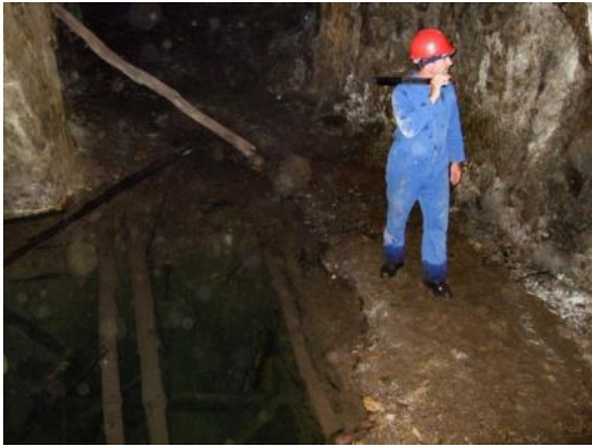
The interior of the mine is wet. The horizontal adit is ankle deep in water, even in summer. There are unprotected, water-filled vertical shafts in the floor of the main mining chamber.
